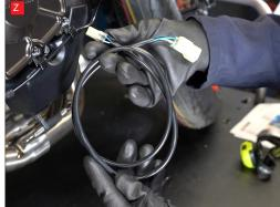
Y) Note the route the wiring runs, then remove the sensor from the bike. The cable tie around the coolant hose is reusable, do not discard it as you will need it later.
