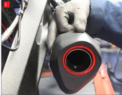
I) Looking from the rear of the bike ensure the silencer does not protrude past the foot peg.
