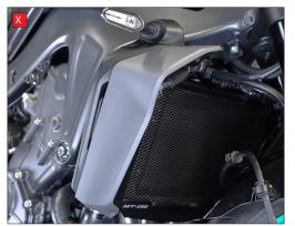
Q) Carefully un-clip and remove the plastic panel.
