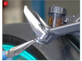
I) Align the bracket with the mounting point on the bike. Use the original mounting bolt to secure in place but leave slightly loose at this point to allow for some adjustment later.
